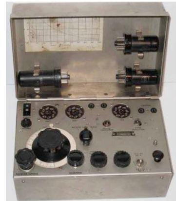
The so-called ‘Para set’ (or ‘Cash box’) version to the right would have to include a separate transformer. The valves - here clipped in the lid have to be stood upright.
